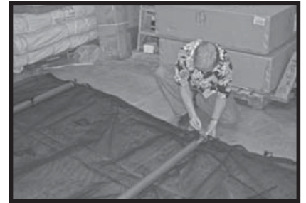
9- Using (2) additional poles, repeat steps 5-8 twice more, using the straps located on the upward side of the mesh.
