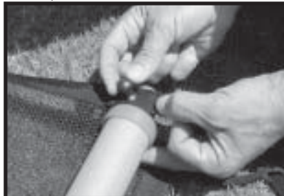
8- Insert pole cap bolt as shown and secure with nut.
